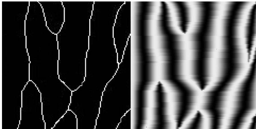
**Fig. 10.** The image on the left shows one example of random corrugation peaks, and the image on the right is the resulting grayscale template.
